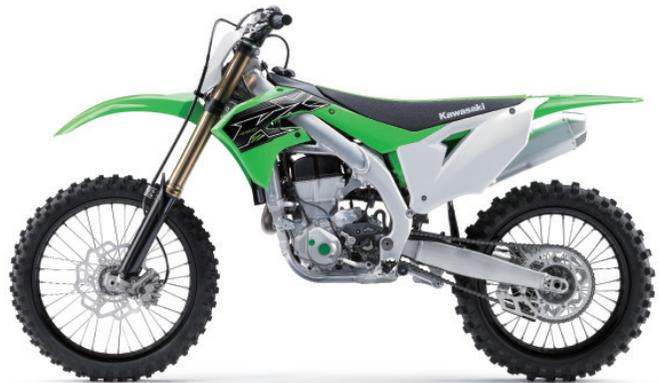
The engine of the KX450 has always been strong, and the lightweight engine package is even stronger in 2019 thanks to the input from Kawasaki's factory race teams. The four-stroke, single cylinder, DOHC, water-cooled 449 cc engine has increased peak power and a flatter torque curve that makes it easier to get on the gas sooner.
